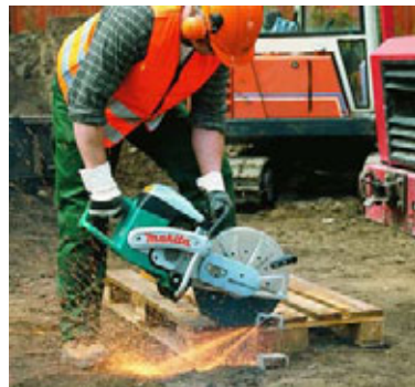
Makes light work of trimming steel girders to length and cutting construction steel.
