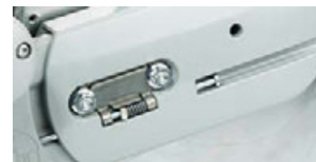
Simple knob adjustment of blade guard. Tension of drive belt easily adjusted with a screwdriver. Marking provided for instant visual check on correct belt tension.
